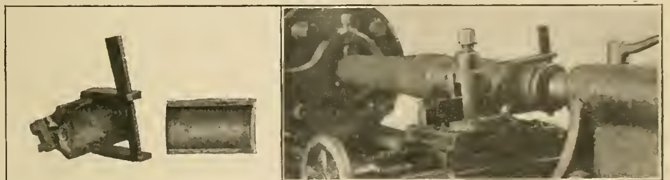
VIEW OF THE FILLET TOOL IN ITS GUIDING SHELL AND METHOD OF APPLYING IN THE LATHE.
